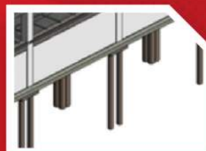
5 PONDASI BORED PILE
